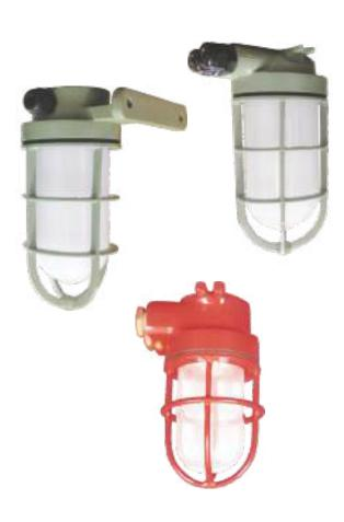
Die cast Aluminium body with die cast protective wire guard with U-shape polycarbonate milky shade with rubber gasket, 2 way connector with 2 cable entries and PG cable glands. Stainless Steel hardware. Fitting for 12W. 240V. LED with Suitable Electronic LED Driver. Fitting in the line of IP 65 protection.
